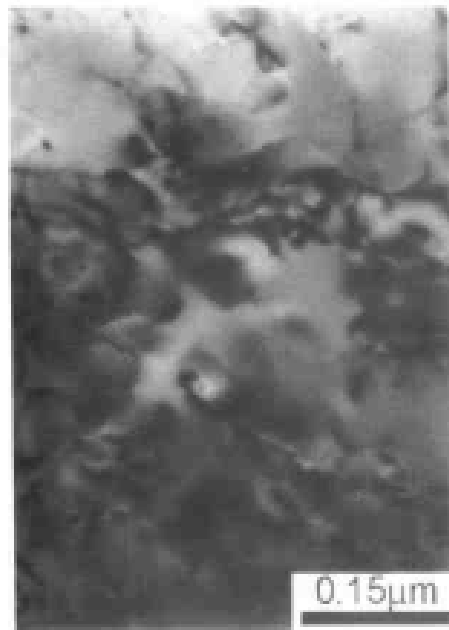
图4-29 激光熔覆,铝基体,镍熔覆材料,YAG激光,TEM照片,显示铝中的位错,扫描速度2.5mm/s,脉宽4ms,频率8Hz,功率密度 5.36 \times 10^8 \text{ W/m}^2 Laser coated Al with Ni, TEM micrograph, showing dislocations in laser coated Al, scanning speed 2.5mm/s, pulse width 4ms, frequency 8Hz, power 5.36 \times 10^8 \text{ W/m}^2 .
