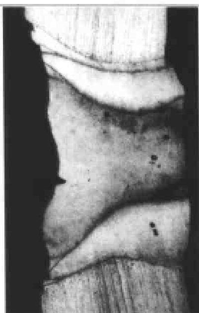
图 5-25 5754 铝合金, YAG 激光焊对接接头横截面金相照片, 板厚 1mm, 60 \times 5754 Al alloy, YAG laser welding, metallograph of a cross butt joint, thickness of plate 1mm, 60 \times .
