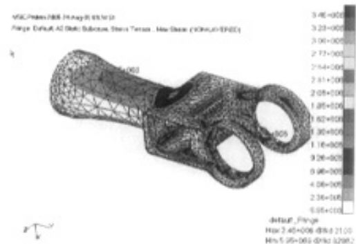
图 3-4 改进后小臂剪切应力分布图 Fig.3-4 Distributing of shear mises in the redesigned small arm
