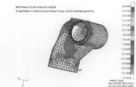
图 3-10 转座剪切应力分布图 Fig.3-10 Distributing of shear mises in the rotated base
